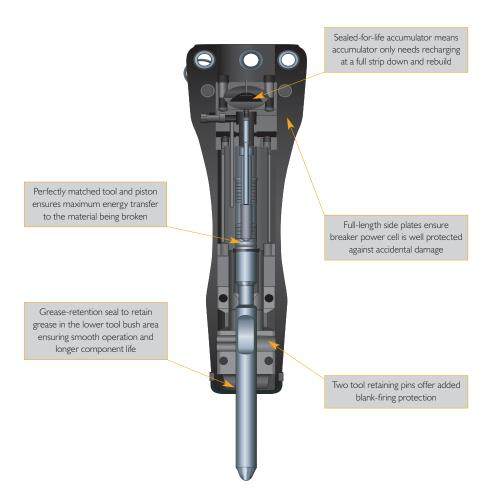
Hydraulic accumulator gives greater acceleration in the power stroke and reduces pressure peaks in the carrier hydraulic system.
