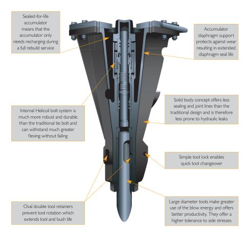
Well-protected charge point reduces the possibility of damage during operation.
